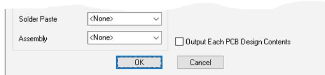
By selecting the **Output Each PCB Design Contents** check box, a copy of each of all the PCBs in the panel are exported. With it not selected, only the contents of one PCB is exported.
