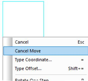
This can be used when an item is copied and after paste. This will cancel the move of the item and release it back in its original position.
