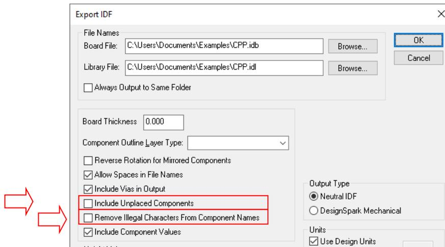
**Remove Illegal Characters From Component Names** - check this box to remove characters that are illegal in Component names for some programs, such as Inventor 3D. They will be replaced with an underscore. These characters include: \, /, :, \*, ?, ", &gt;, &lt;, |
