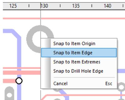
There are options on the context menu to snap the ruler stop to the item you finish on. The snap to origin, extremes and drill edge work the same as the existing options from the ruler bar. The snap to item edge option will snap to the closest edge on the item.
