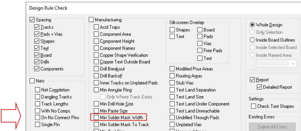
The minimum mask to track value can be set in the **Design Technology** under **Rules** and **Solder Mask**.
