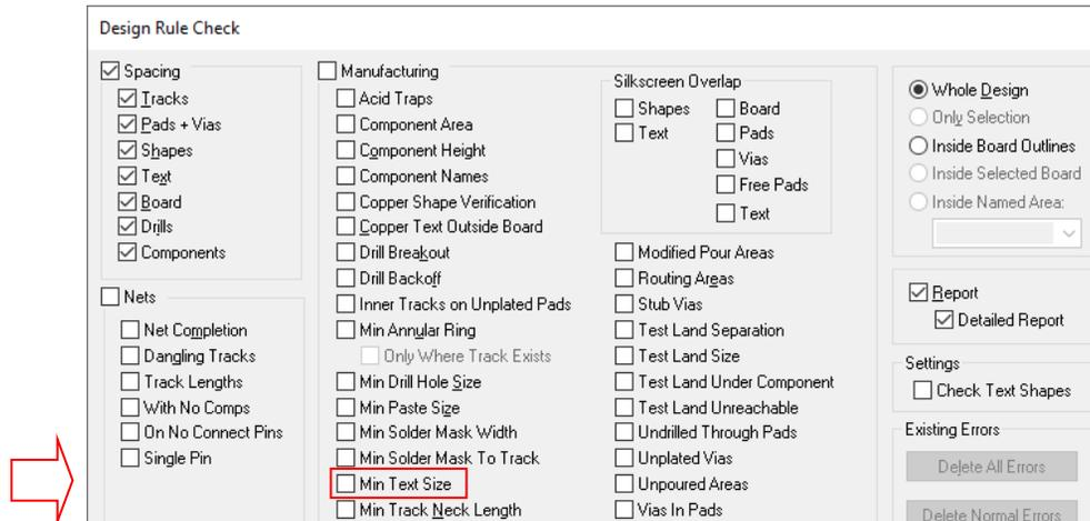
The min text size is defined in the **Design Technology, Rules** dialog on the **Settings** menu. Defining and running this check will ensure that all text added to your design is manufacturable, for example, copper or silkscreen text.
