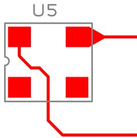
Likewise, once the teardrop is added, you can select the pad and remove the teardrop using the **Remove Teardrop from Selected Pad** option.
