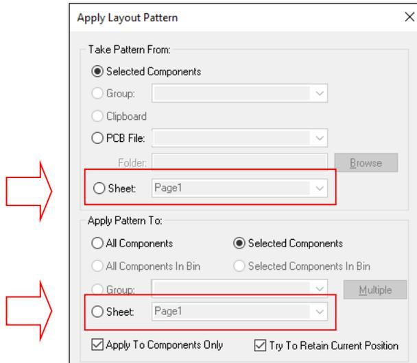
Select an existing Schematic design sheet from the **Project**. If the PCB was created without a project, only one sheet name will be available.
