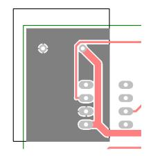
Copper Pour Areas are not plotted and will not appear on your plots, they provide the system with an intelligent area into which the copper can be poured.
