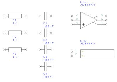
Before we add the connections, we should change the component values to be the ones required. This is easy to do because we've used 'generic' components. If you prefer to use specific Parts, you can also work this way with Easy-PC.
