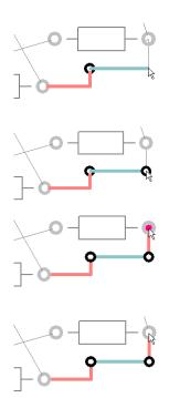
A via has been added automatically and the track layer is now on the Bottom side and is shown in a different colour (blue).
