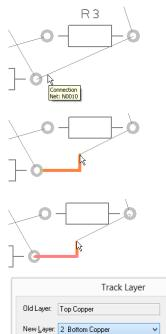
Wires 1 Top Copper Hover the cursor over the connection to reveal the design tooltip. This will tell you that you have selected the correct connection.
