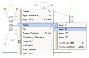
For our design, no mirroring (Flip) will be required. The placement and overall connection lengths could be improved by rotating some of the components. If you feel you would like the practice placing components, select a component and click **R** to rotate it. Component names can be rotated back to be a readable direction separately using the same pick and rotate method.
