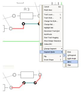
This mode can be changed by accessing the routing mode during routing. Select the **Segment Mode>** from the shortcut menu and choose the mode from the choice of five available.
