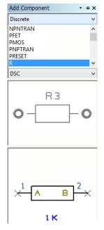
From the list, select the component  $\mathbf{R}$ . Either scroll down using the slider bar or pick in the list and type R, the list will then automatically scroll down to the first component starting with the letter R.
