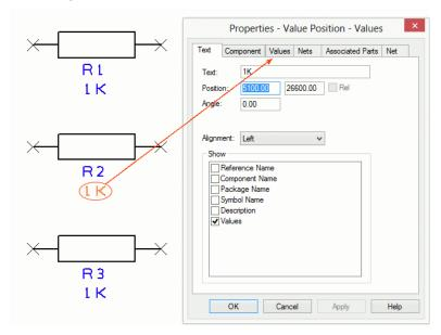
The **Value** field shows the current 1K value and is already highlighted blue. Simply click the **Edit** button or double-click the blue highlighted field to edit the value required. Type in **11K**.
