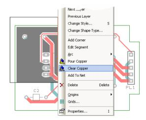
When using poured copper remember you shouldn't use Delete but should always use Clear Copper. Copper Pour Areas can be modified at any time and the area re-poured using the option from the shortcut menu. If you wish to completely remove the copper and area, you must use Clear Copper first and then delete the area afterwards using the Delete key.
