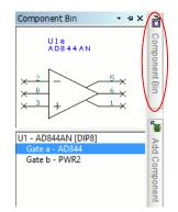
Our Op-Amp (U1) is shown in the Bin as two gates (Gate a & Gate b). Click on **Gate a** under the word **U1 – AD844AN {DIP8}** to see a preview of the symbol above it.
