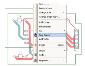
A dialog is displayed from where you can select parameters for the poured area, such as the net name association and thermal connections etc.
