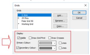
You can also make the grid dots displayed as **lines** on the design. Use the **Lines** check box next to the **Primary** or **Secondary Colours**.
