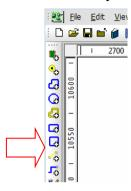
2. Choose a starting point on a grid dot, hold down the left mouse button drag a rectangle down to create a shape 200.00 x 400.00 thou.
