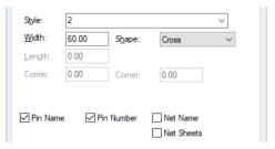
By default, the pin styles is taken from the **Setting** menu, **Defaults** and **Pads**. Pad styles are defined in the Pad Styles dialog under Design Technology.
