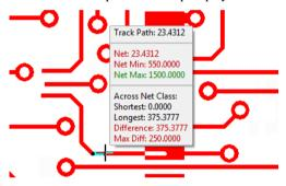
If minimum and maximum track length rules are defined on the net class of the track being edited, their values will be included in the display and will be drawn green if the net track length is within the defined limits. If the net track length is outside one of the limits it will be drawn with red text as well as the rule that failed.
