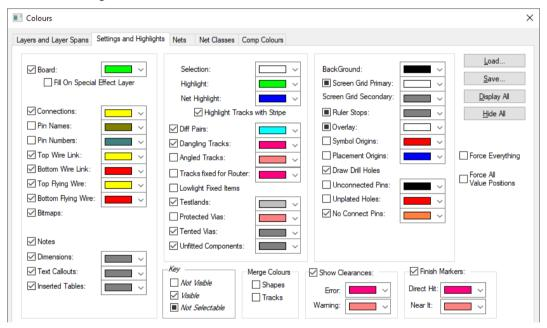
On the **Settings & Highlights** dialog you can also make non-layered items non-selectable by using the tri-state check boxes. The tri-states are unchecked (Not Visible but Selectable), checked (Visible and Selectable) and checked/greyed (Visible but not Selectable), these are shown on this dialog under Key.
