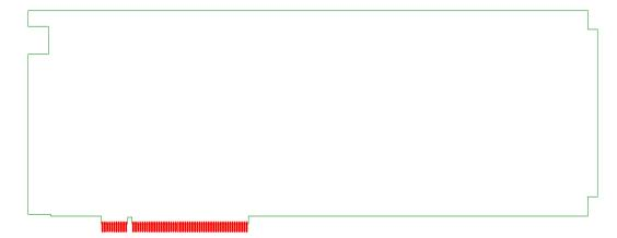
You can create board outlines in a number of methods. You can use the Add Board option to simply create the shape or you can use the **Import DXF** option to use an existing shape created in a mechanical package such as AutoCAD where the shape maybe very complex.
