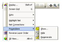
**Show** displays a dialog allowing the selection of which power plane to view. If only one power plane is present in the design, it will not display this dialog but go straight into the display of the power plane.
