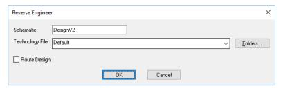
Where a PCB design has been created, and if the PCB design is used to create 'local' libraries with the Schematic symbols added to the components in the new library, you must update the components into the PCB design first before using the Reverse Engineer option. Use the **Update Component** option from the **Tools** menu.
