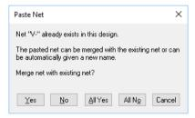
Once a net name is detected, you are prompted with the question - Merge net with existing net? Using the options on the dialog, you can elect to add the net name to the existing net or to automatically allocate a new name to it, therefore not connecting it into the existing net.
