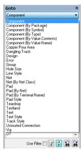
The **Goto Error** selection will show all the design rule errors in the design once the online DRC or batch Design Rules Checking options have been run. Clicking on any of the errors will 'pan' the display to the selected error. Errors can be sorted by **Type** of error and **Layer** of the error using the context menu in the window.
