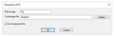
By setting up this dialog, this will give you the name of the PCB design, the Technology File and whether or not to use the Component Bin.
