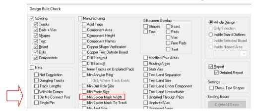
The minimum mask to track value can be set in the **Design Technology** under **Rules** and **Solder Mask**.
