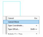
This can be used when an item is copied and after paste. This will cancel the move of the item and release it back in its original position.
