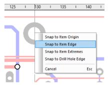
There are options on the context menu to snap the ruler stop to the item you finish on. The snap to origin, extremes and drill edge work the same as the existing options from the ruler bar. The snap to item edge option will snap to the closest edge on the item.
