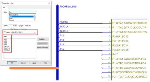
When starting or ending a **Bus** on the segment of an existing **Closed Bus**, it will now inherit the **Net Name** and **Bus Name**.
