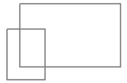
The **selected** shape with the largest area is used as the 'parent' shape, and all the other selected closed shapes that overlap with this parent shape are used to make cutouts of the outer shape. The original 'inner' shapes are then deleted.
