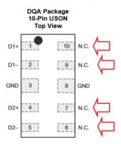
To help ensure that these are not accidentally connected in your design, a pin in a Component can now be marked as **No Connect**. This status is applicable to both Schematic and PCB designs.
