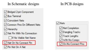
**Translate to PCB** and **Integrity Check** will also report warnings about **No Connect** pins in the Schematic that have nets assigned to them:
